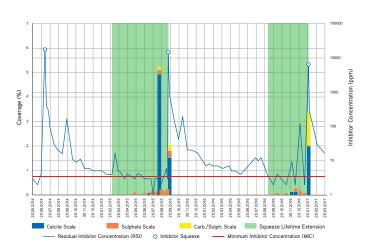
BSA™ analysis of the amount and type of inorganic scale used for scale squeeze lifetime extension.
