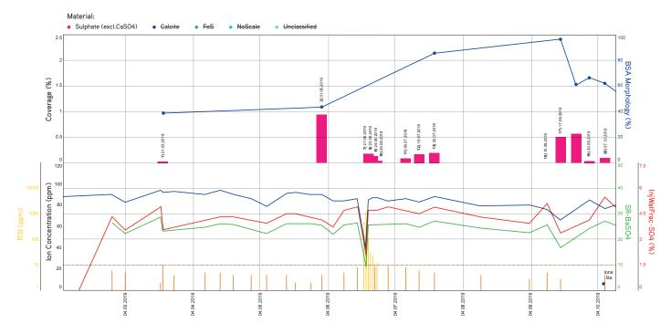
Example of ScaleMan software capabilities. Sulphate scale coverage and morphology trend plot combined with trends for ion, injection water fraction, scale potential (SR), residual inhibitor concentration (RSI) and minimum inhibitor concentration (MIC).
